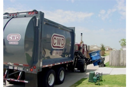
Automated side load recycling vehicle servicing Single Stream recycling cart
