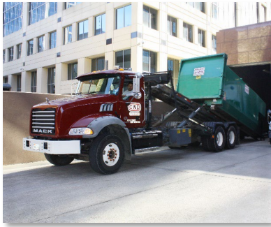
35 yard self contained compactor being serviced by CWD roll-off truck
