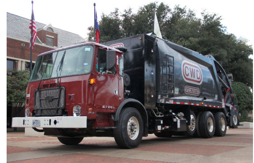
Rear Load CNG and DOT weight certified
