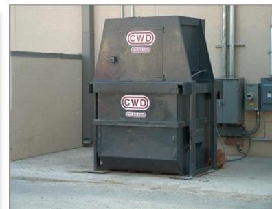
6 cubic yard front load compactor
