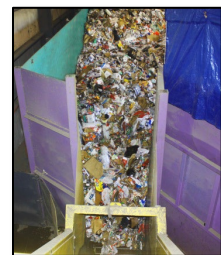
Recyclables traveling up the first conveyor
