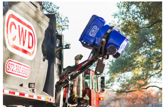
Automated Side Load (ASL) service
