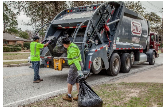
Rear Load hand collected trash and 95-gallon cart recycling.
