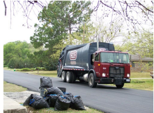
Rear load vehicle facilitates hand load collection
