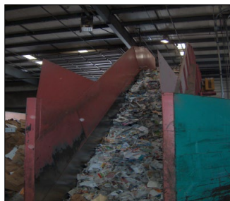
Newspaper traveling up the conveyor to be baled
