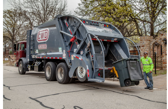
Rear Load hand collected trash in 95-gallon carts
